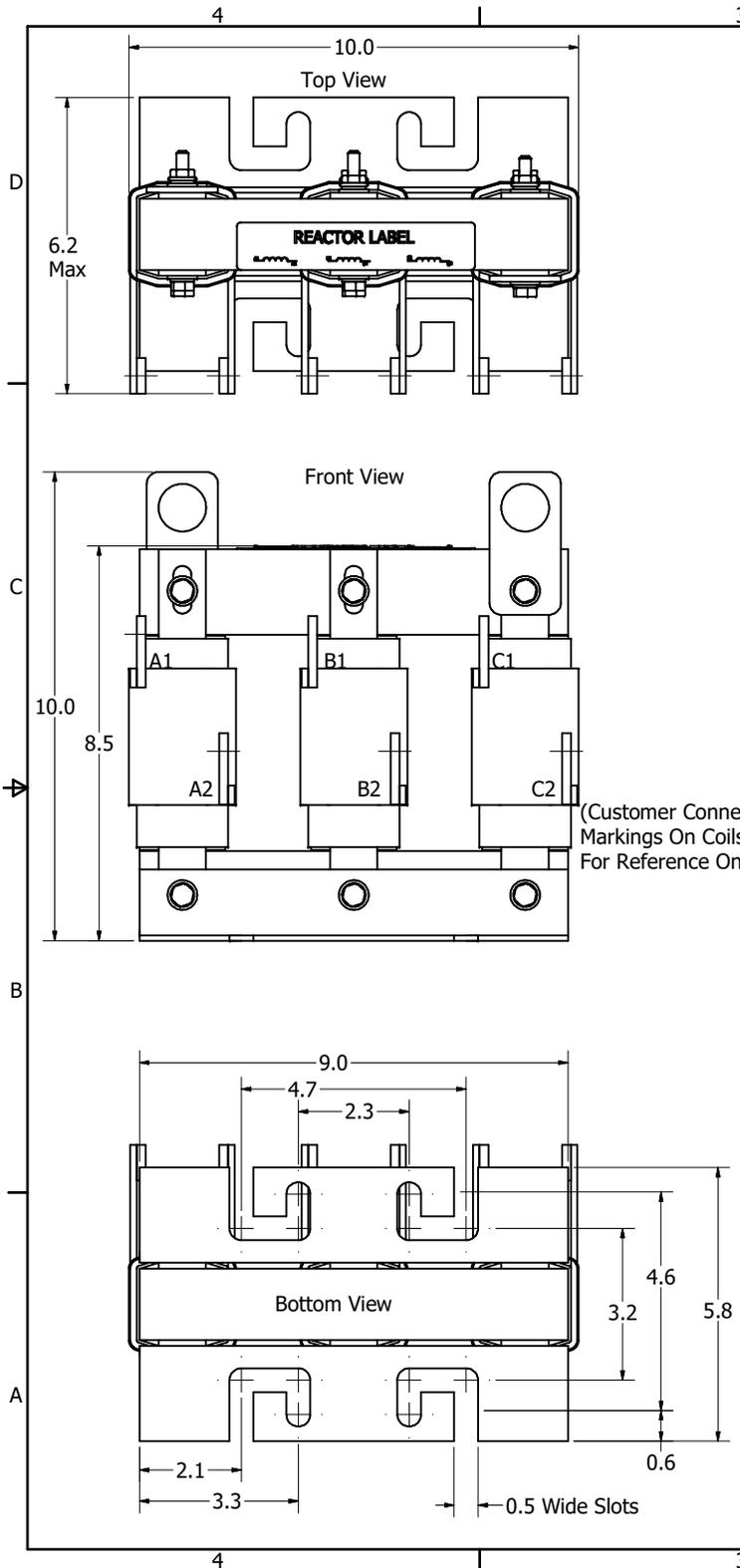
208/240 Rated Voltage, 600 Max Voltage, High Z, Impedance.
