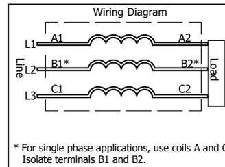
\* For single phase applications, use coils A and C, Isolate terminals B1 and B2.
