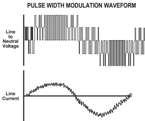
Figure 1 PWM Waveform
